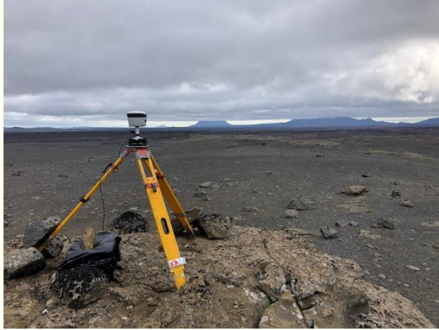
Fig. 6 Installed Trimble GNSS base station
