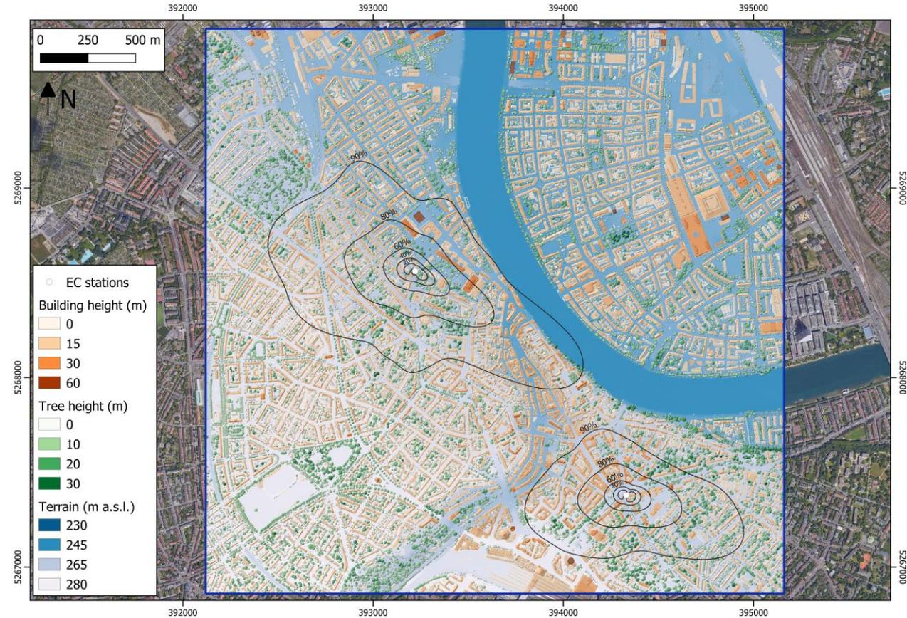
Figure 4. Building, tree and terrain height maps of the study area. The average turbulent flux source area isopleths for 2017-2018 are displayed for the two urban EC stations.
