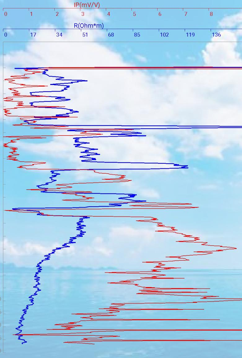
The resistivity curve (R, blue) is recording the apparent specific resistivity of the media. In sand and clay mix the higher values caused by sand and fresh water.
