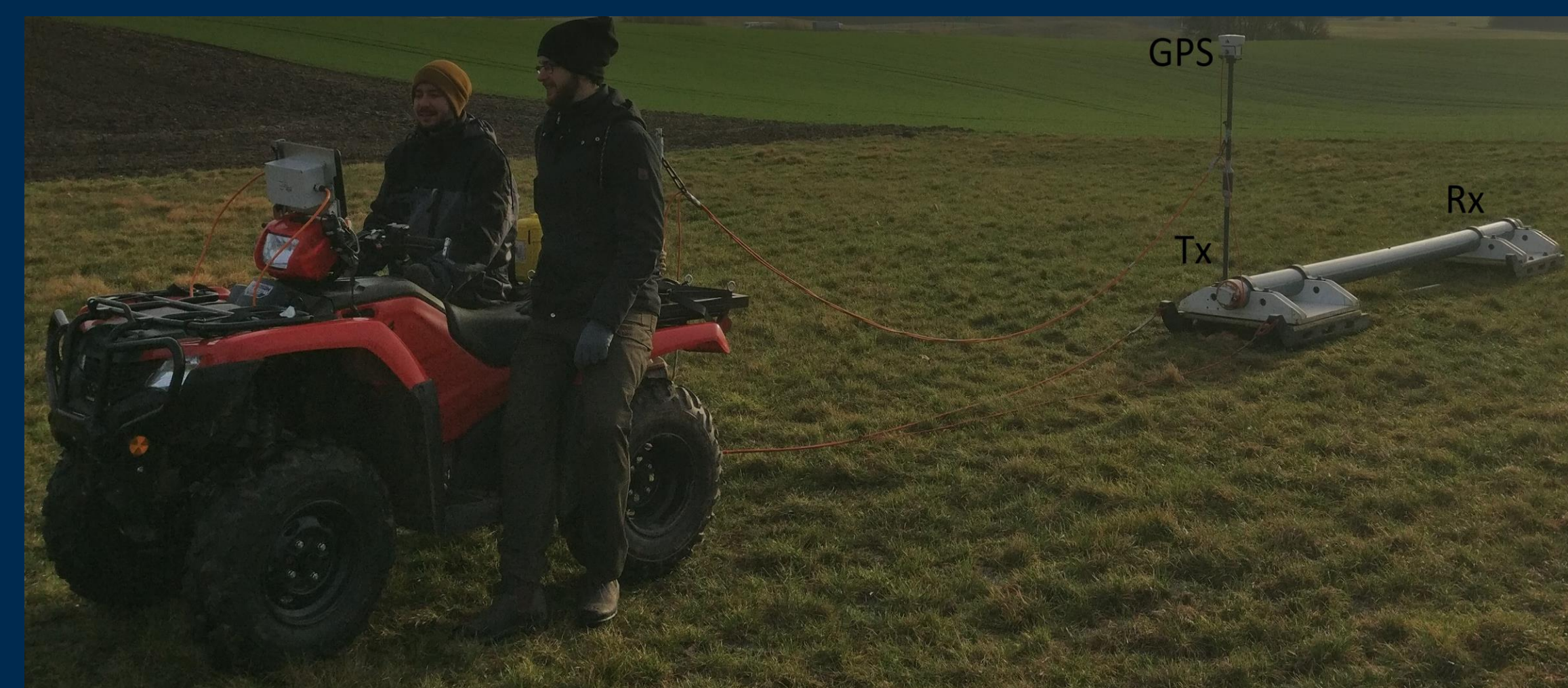
Figure 1. A sledge mounted EMI instrument towed by an all terrain vehicle. The tube contains the transmitter (Tx) and receiver (Rx) coils and a GPS is mounted on the sledge.
