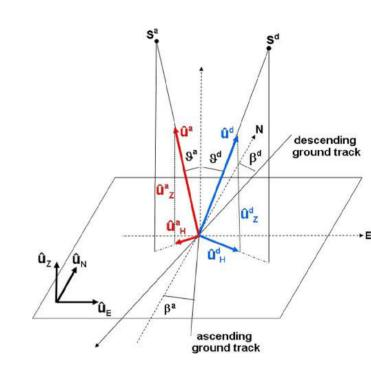
Sketch with the geometry of ascending and descending InSAR geometries with unit vectors (red)  $u^a$  and (blue)  $u^d$ , radar incidence angles  $\vartheta^a$  and  $\vartheta^d$ , and angles  $\beta^a$  and  $\beta^d$  related to ground-track azimuthal angles. The horizontal components of unit vectors  $u^a$  and  $u^d$  are also depicted (after Catalao et al., 2011 and Vassileva et al., 2017)
