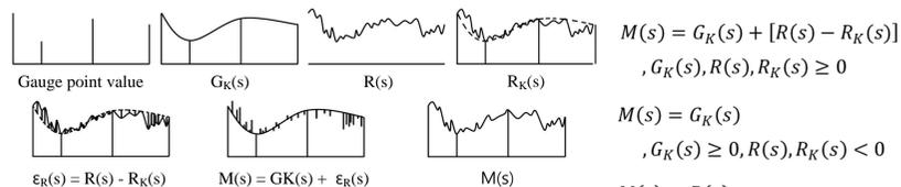
Concept of the conditional merging method (modified from Sinclair and Pegram, 2005)
