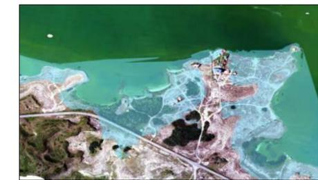
Areas of potential inundation after planned rise in water level of Lake Sevan modeled from UAV-derived highly-detailed DSM
