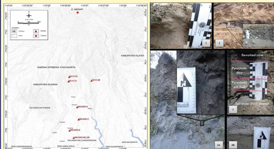
Left: Map of the location of the ash samples (After Seraphine, 2018). Right above: Photos of the outcrops from which samples were collected (After Seraphine, 2018). Right below: Photo of the Fourier-transform infrared spectroscopy configuration in Natural History Museum of Stockholm (Image courtesy of B. Radu, Natural History Museum of Stockholm)
