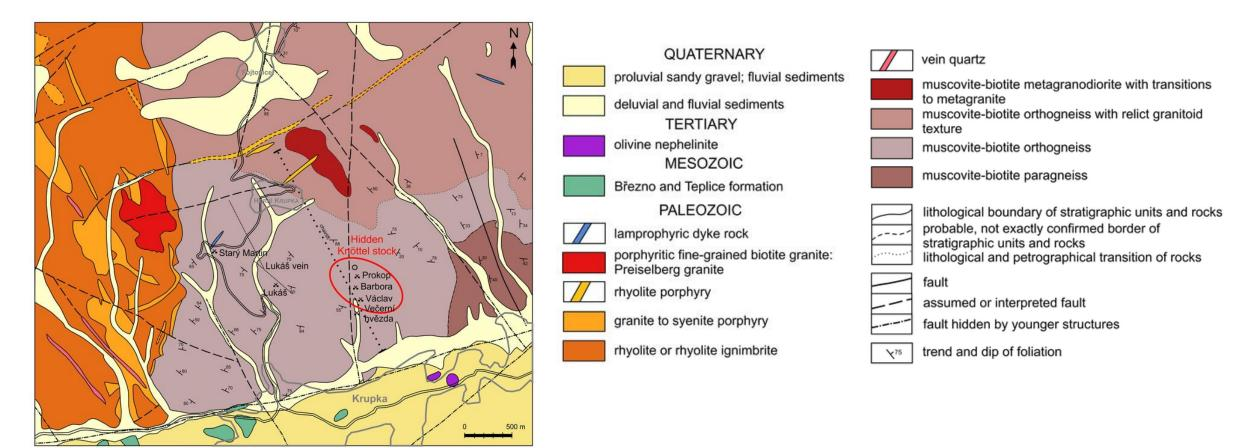
The granite-pegmatite-greisen stock belongs to the series of minor shallow-level intrusions (327-317 Ma), emplaced near the contact of the Teplice-Altenberg volcanic complex (caldera) with the pre-Variscan metamorphic complex (two-mica gneisses)
