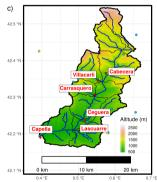
Thin black lines outline subbasins, red triangles mark the position of discharge gauges, blue and green points show gauges of rainfall and other meteorological variables, respectively.
