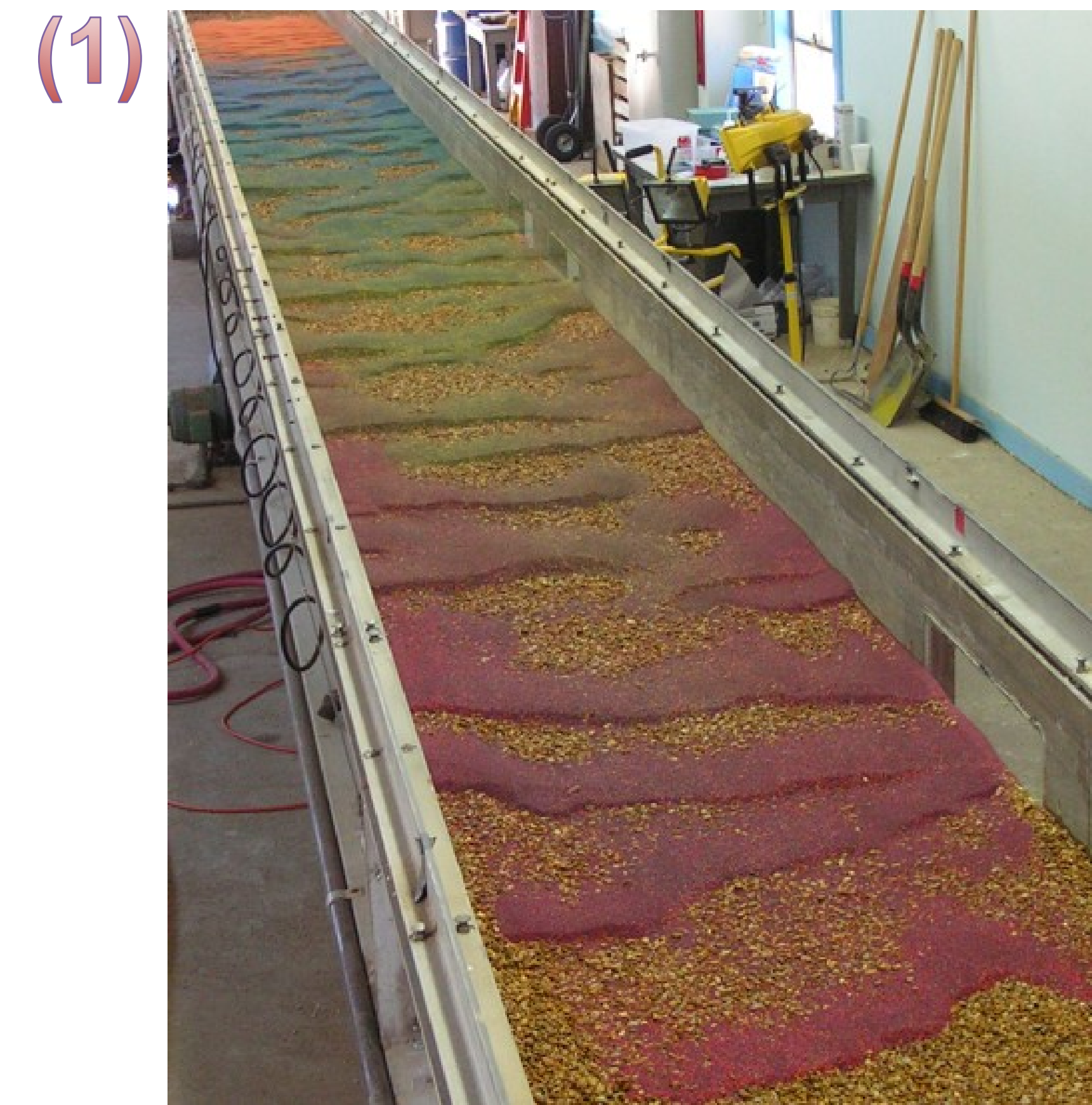
(1) Flume experiment with different-colored sand particles. Flow was from top to bottom of photo.
