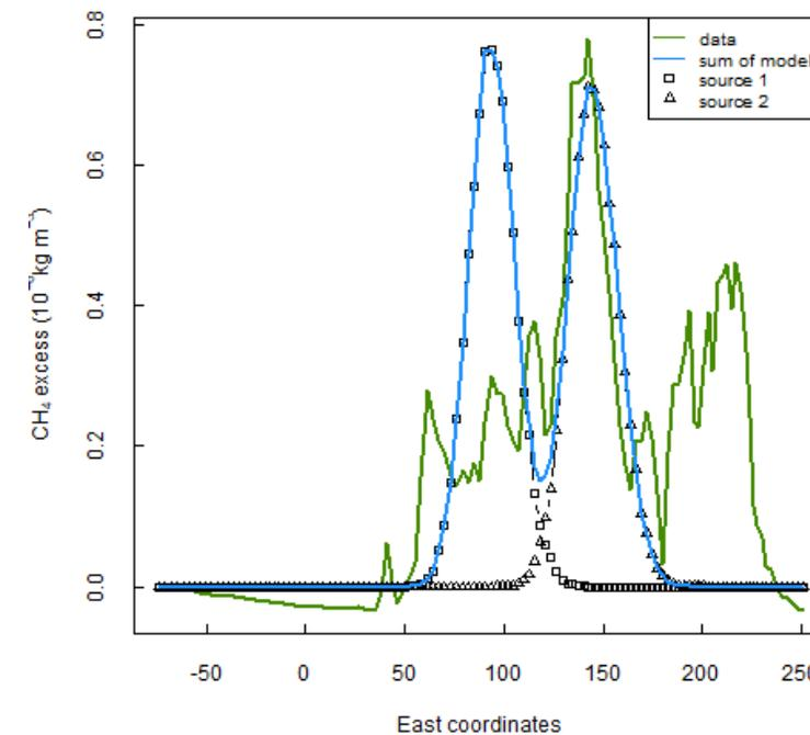
Collected data were analysed with R codes written by J. Kammerer. Typical for this farm is a double peak, which is due to two sources, namely the farm and the close by biogas plant. Emission estimated for this farm (320 cows) equals  $2.6 \pm 0.7 \text{ g CH}_4/\text{s}$ .
