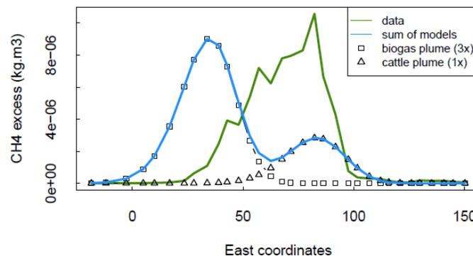
Estimated emission for the first 8 peaks equals  $4.1 \pm 1.3$  g/s. For the next 12 peaks (with higher wind speed) emissions equals  $24.5 \pm 10.9$  g/s. In the second case the estimated emission is much higher than from January 2020. It is more complicated case, because wind speed has increased.
