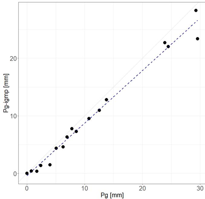
For 2019, 9 of the total 22 measurement weeks, the grass was short and left the grids uncovered. This data suggests that the grids captured well up to 30 mm precipitation per week.
