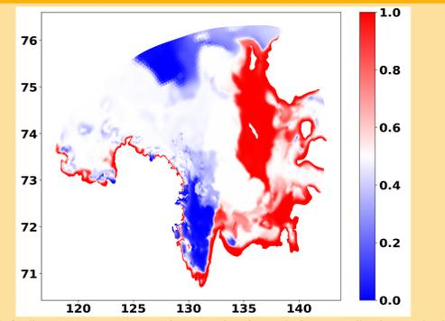
Figure 7 Sediment transport experiments showing relative contribution at bed from coastal (red) or river (blue) sediments. Due to the offline coupling issues this has been run online so has not yet been run long enough to get equilibrium
