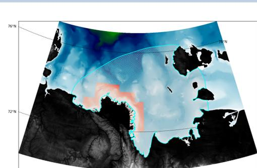
Figure 1: Laptev sea FVCOM model with bathymetry.
