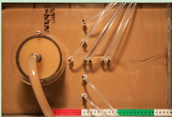
In a **laboratory setting**, several sand samples were mixed and subjected to a hydraulic head difference between an inflow filter on one side and a **single exit point on the top** of the experiment. As the top of the experiment was see-through the **progress of the pipe could be monitored visually** (left). The results of this experiment are used to calibrate a digital model (right). **See the QR code for an animated version**
