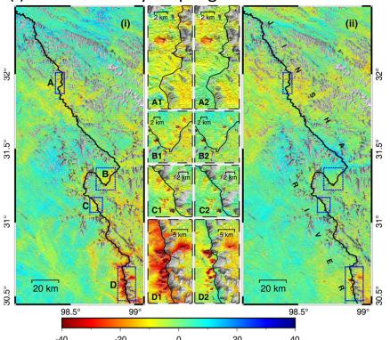
The mean deformation rate map along the Jinsha River by InSAR stacking (i) without and (ii) with atmospheric correction.
