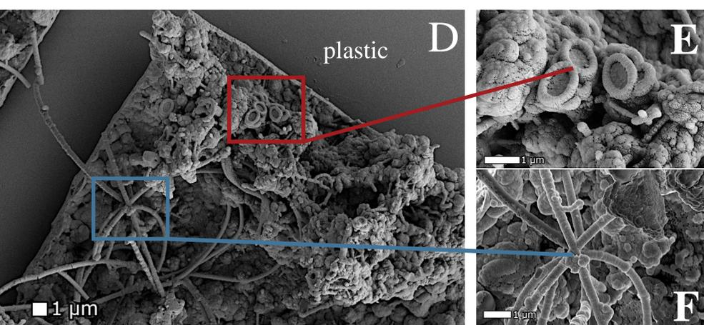
SEM images of D) biofilm developed on PS floating at the sediment water interface for 6 months. E) high diversity in biofilm F) mineralized *Lyngbya* sp., an ubiquitous autotroph in the Øresund or a sheath structure. EDS analysis on highlighted spots in E and F were enriched in Fe and Cr, possibly indicating a Fe and Cr-rich coating.
