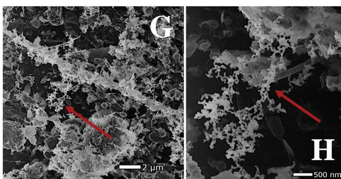
He Ion microscopy images of PE exposed to surface sediments for 10 months. Potential iron minerals secreted by iron reducing bacteria. (personal communication, S. Chiriav, MCI, NanoSyd-SDU)
