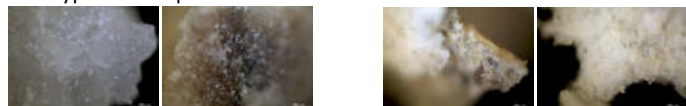
Figure 3: OM, dark field, 10x. The white crust samples present some translucency grains, although visually distinct. Efflorescence samples present similarities in hue, heterogeneity and grain size.
