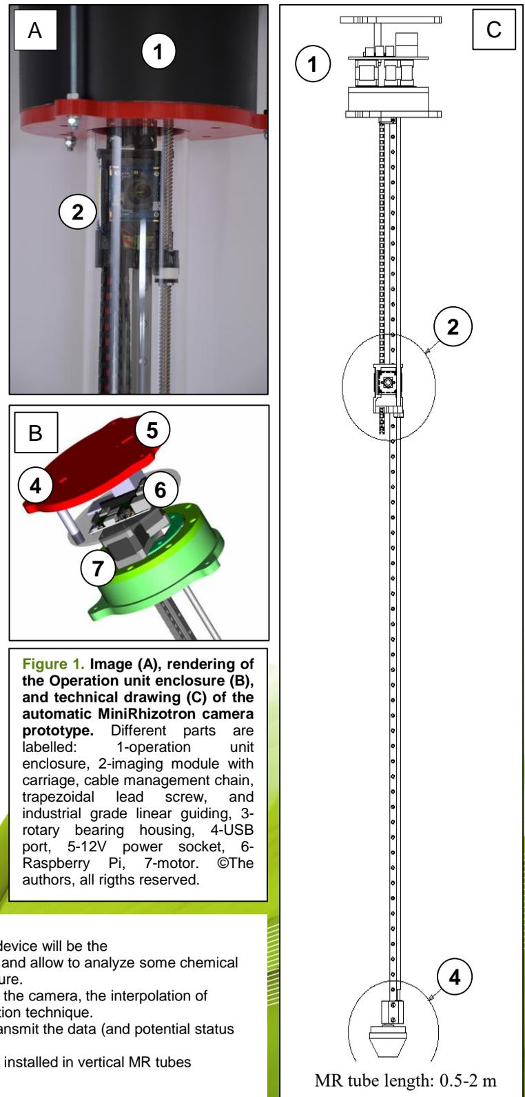
**Figure 1. Image (A), rendering of the Operation unit enclosure (B), and technical drawing (C) of the automatic MiniRhizotron camera prototype.** Different parts are labelled: 1-operation unit enclosure, 2-imaging module with carriage, cable management chain, trapezoidal lead screw, and industrial grade linear guiding, 3-rotary bearing housing, 4-USB port, 5-12V power socket, 6-Raspberry Pi, 7-motor. ©The authors, all rights reserved.
