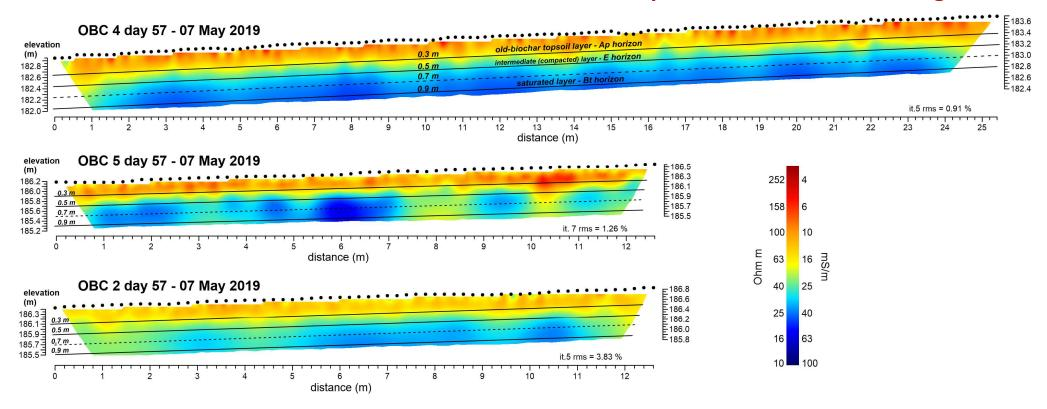
ERI characterization of 1 m thick soil profile at OBC 2, 4 and 5 monitoring zones on day 57 (07-May-2019). Inverted resistivity values at 0.20, 0.45, and 0.80 m depth all along the transects were extracted and converted to conductivity,  $\sigma_b$ , adjusted at T = 25 °C and averaged at each depth afterwards,  $\sigma_{b,25}$ , for its analysis. Similar results of inverted ERI sections were obtained during the whole monitoring campaign not shown here for simplicity
