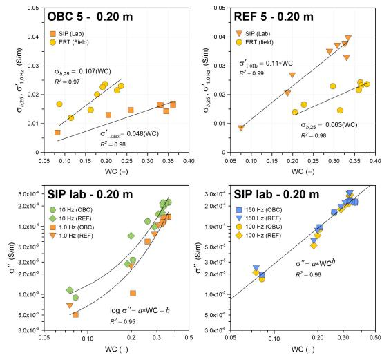
**Top panel:** correlations between  $\sigma_{b,25}$  (field-scale),  $\sigma'_{1Hz}$  (lab-scale) and WC at 0.20 m depth in OBC 5 and REF 5 zones
