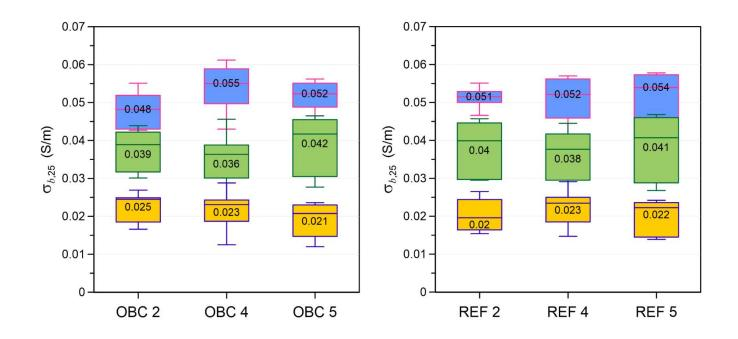
Comparison of median values  $\sigma_{b,25}$  (labels and middle horizontal line) at monitoring depths of 0.20 m (bottom) , 0.45 m (middle), and 0.80 m (top) at each OBC and REF zones; the bars show the minimum and maximum  $\sigma_{b,25}$  values, the color bars show the percentile rage (25 – 75)
