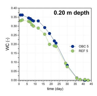
**Left:** water content (WC) variation from controlled desaturation experiment at room temperature in OBC 5 and REF 5 undisturbed soil samples collected at 0.20 m depth in trenches. **Right:** associated phase shift,  $-\varphi$ , and magnitude,  $|\sigma^*|$ , spectra from SIP measurements.
