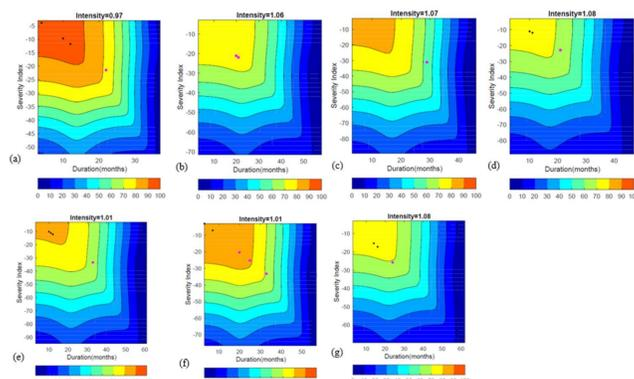
Fig. 5: The joint probabilities of drought events of any duration, severity or intensity of interest based on SPEI-12 for cluster 1 (a) to cluster 7 (g)
