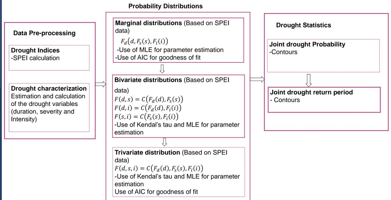
Fig. 1: Sketch of the sequence of methodologies used in this study for drought analysis.
