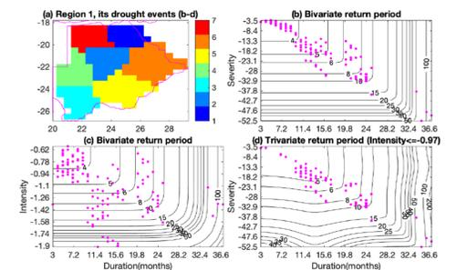
Fig.6: Joint bivariate and trivariate return periods of drought duration, severity, and severity in cluster 1 during 1901-2018
