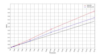
Scalability tested up to 122 000 cores Good scalability up to 50 000 cores Simple precision improve scalability compared to double precision
