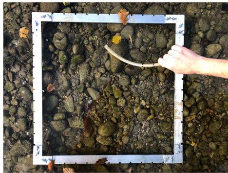
Figure 2: Frame and tube for the application of the Finstad method
