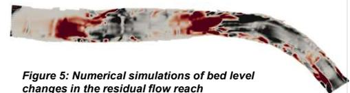
Figure 5: Numerical simulations of bed level changes in the residual flow reach
