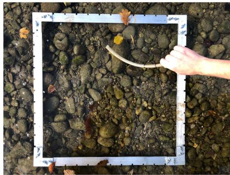
Figure 2: Frame and tube for the application of the Finstad method
