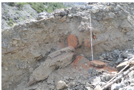
The larch trunks, > 10 m long and up to 60 cm in diameter provided excellent material for dendrochronology. 2 slabs were cut for analyses. (photo Ch. Schlüchter).
