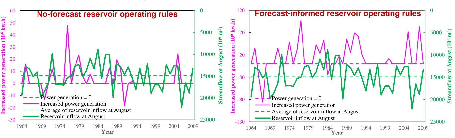
The reservoir operations based on rules selection can increase the power generation in most cases, especially in the years with relatively lower streamflow amount.
