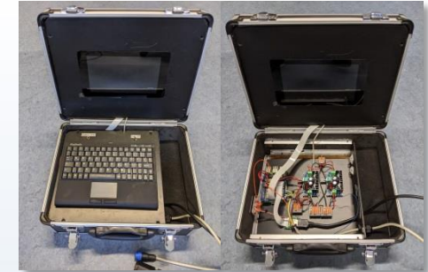
Fig. 3: Raspberry Pi-based control unit containing of a Raspberry Pi 2 model B, an 8" touch-screen, a keyboard, two voltage regulators (5 V and 6 V), and a CSI to HDMI adapter.
