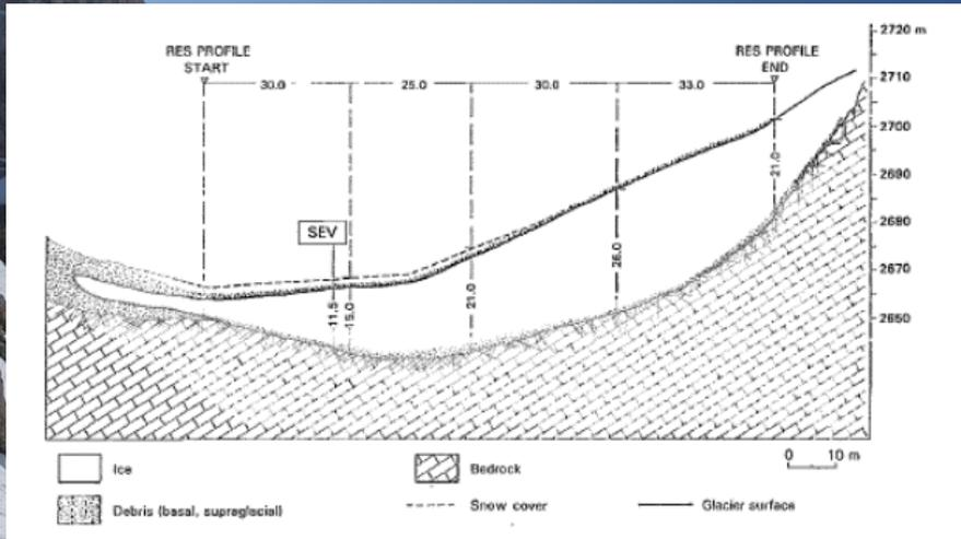
GPR data have been collected since 1990 along and across the main axis of the glacier, in order to estimate the ice thickness below the debris.
