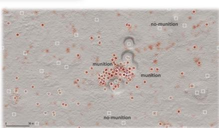
A simple three layer CNN allowed to calculate the probability of a 15x15 cell size tile to contain a munition object (red)
