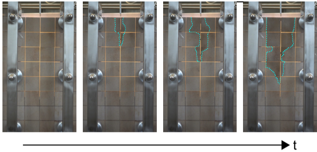
Figure 7: Flow through fracture networks and well-known topology/geometry (Rüdiger et al. 2020, under revision).
