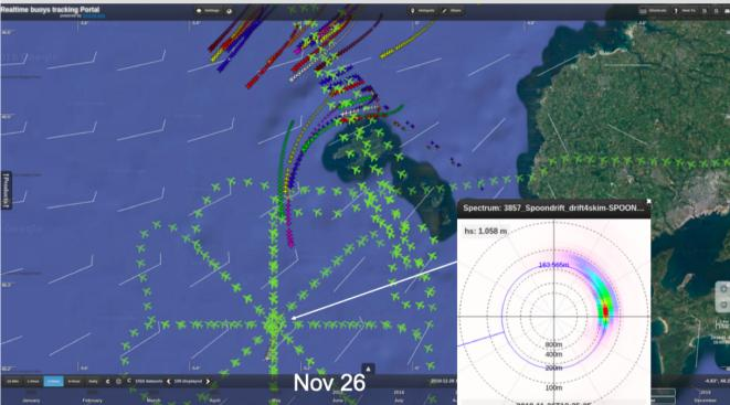
Dedicated online portal has been set up for planning the DRIFT4SKIM campaign, monitoring the deployment in real time and analysing results. This has been useful to adapt the in-situ/airborne colocation in real time.
