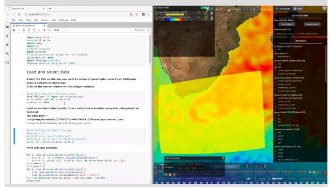
Sea level data are extracted in SEAScope, sent to a Jupyter python notebook. Geostrophic currents are derived from the exported data, analysed and sent back to SEAScope to be compared with other currents or in-situ data.
