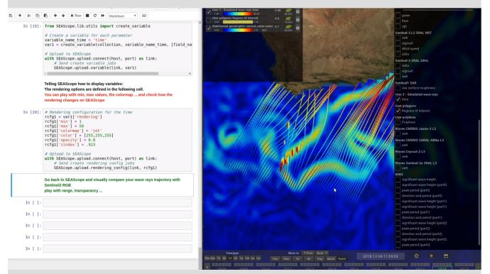
Ocean current data are selected and extracted in SEAScope, used in a Jupyter python notebook to simulate wave current interaction and resulting waves rays are viewed in SEAScope together with contextual datasets.
