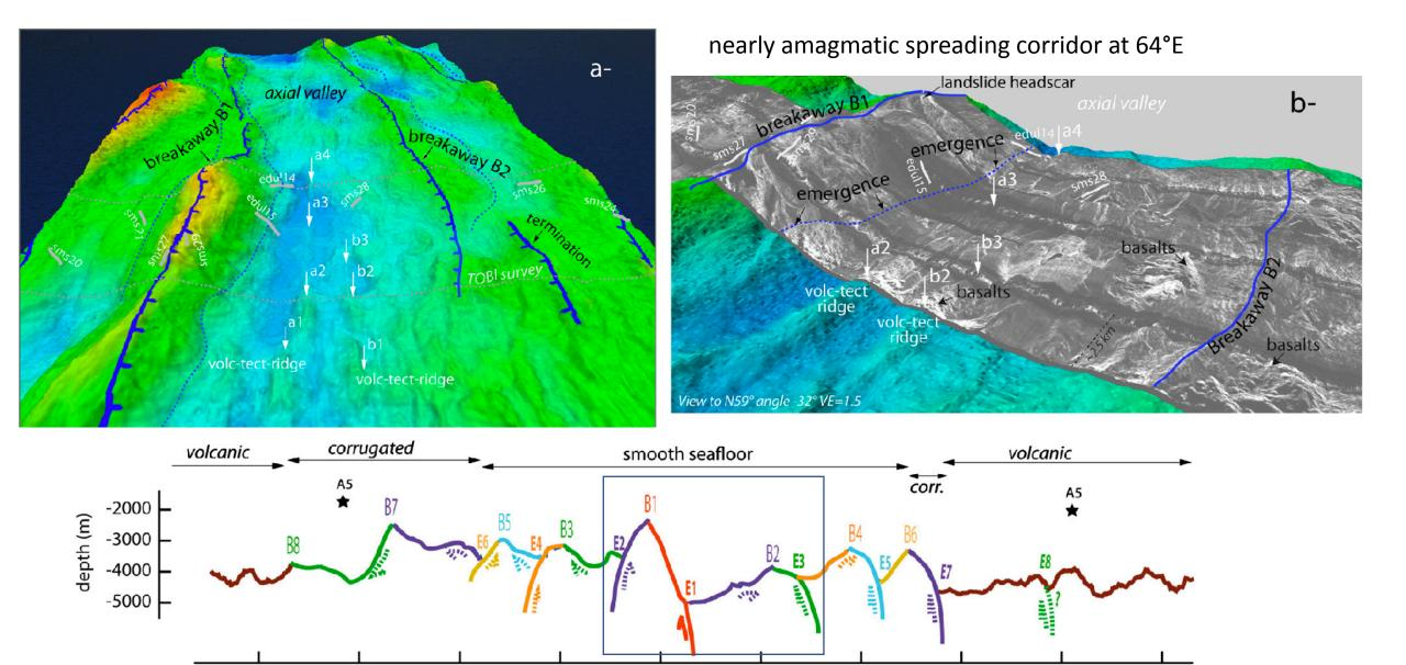
The part of the plate divergence that is not accommodated by magma emplaced as gabbros or basaltic dikes is taken up by normal faults that exhume upper mantle-derived rocks.
