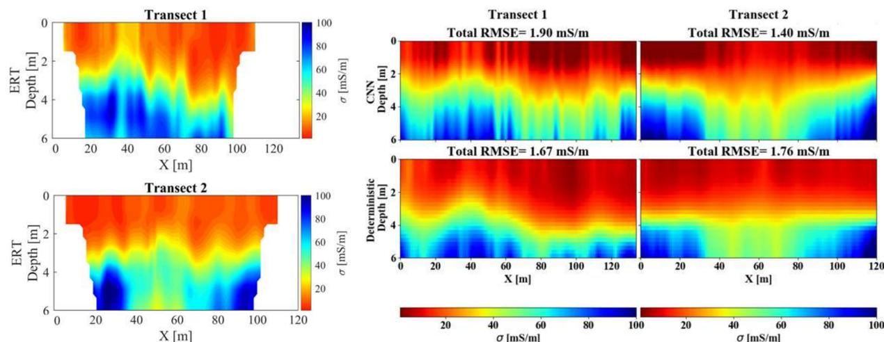
The CNN-derived subsurface EC of both transects match closely with their counterparts from ERT data. The AarhusInv employed vertical and lateral constraint and consequently the deterministic solutions are rather smoother than the CNN results. The RMSE values between the measured and modelled data for all scenarios demonstrate a well performance of both inversion strategies.
