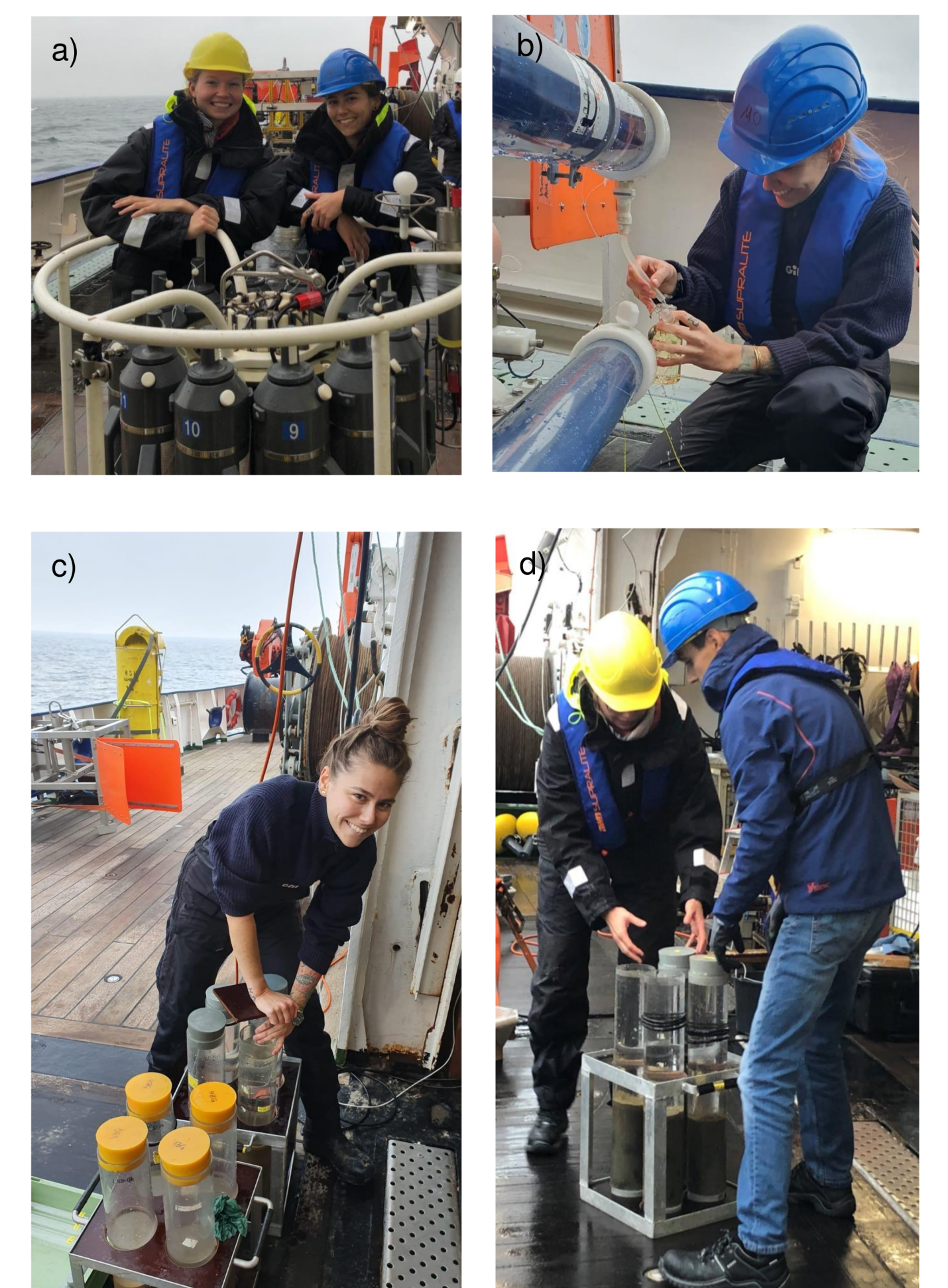
Fig. 3: Photos from cruise HE541 during the sampling: a) with the CTD rosette, b) alkalinity sampling with bottom water scoop, c) cut out mini cores for batch core incubations, d) pore water cores.
