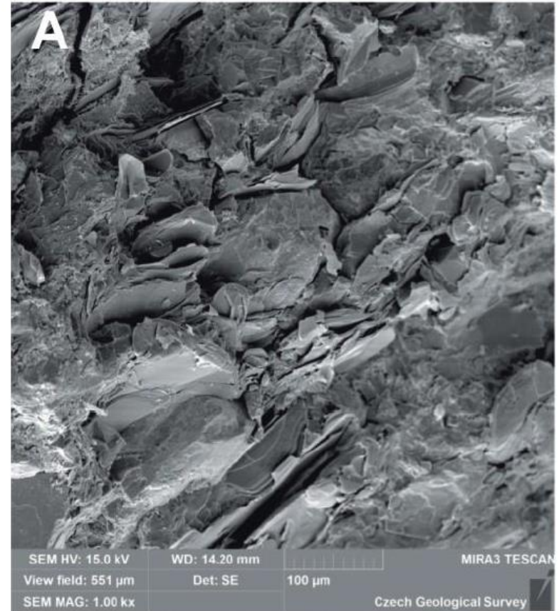
Microphotograph. Graphite leaves are parallel to schistosity.
