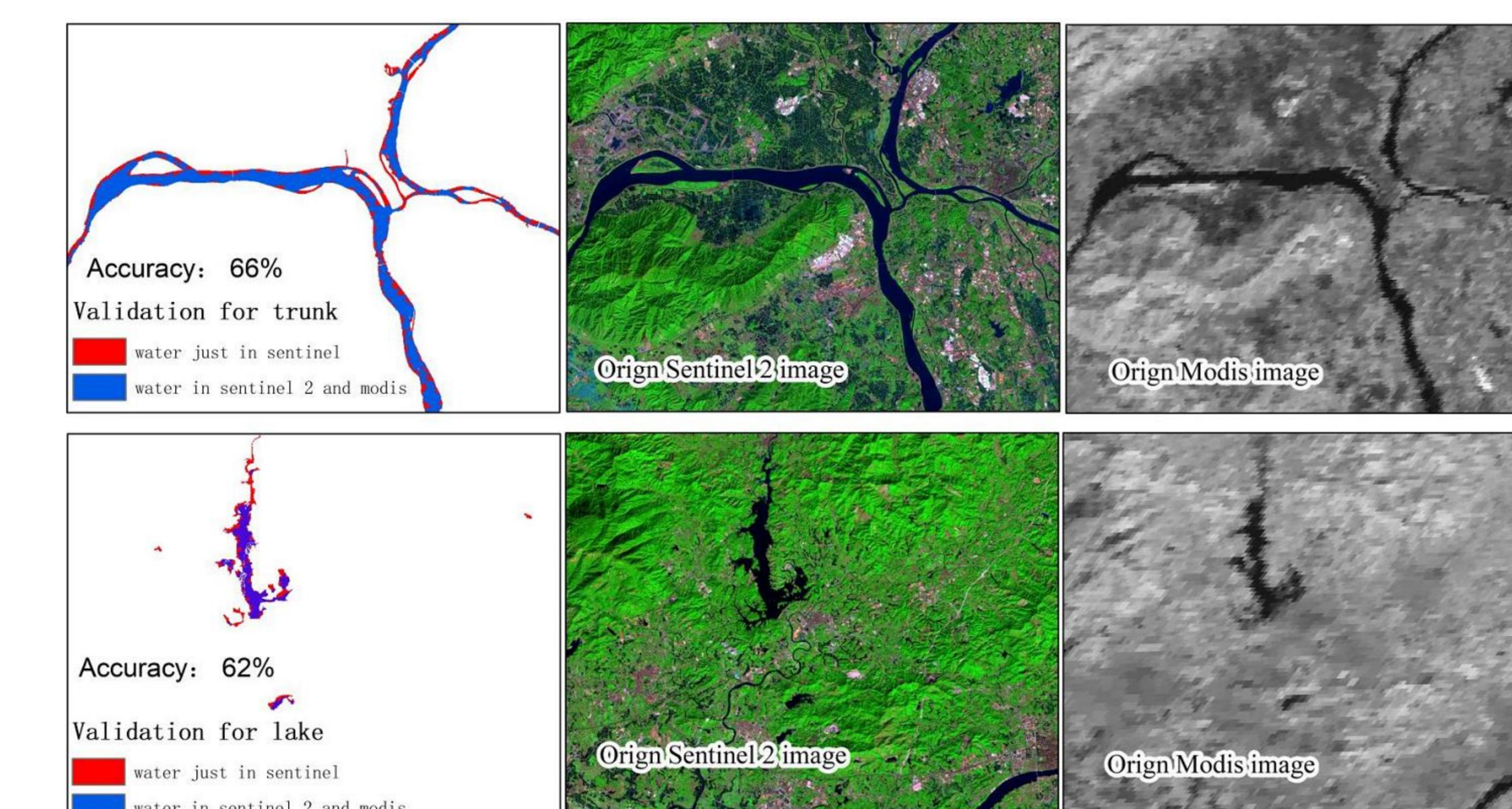
Figure 5 Using Sentinel 2 image validated the accuracy of water body monitoring based on Modis image
