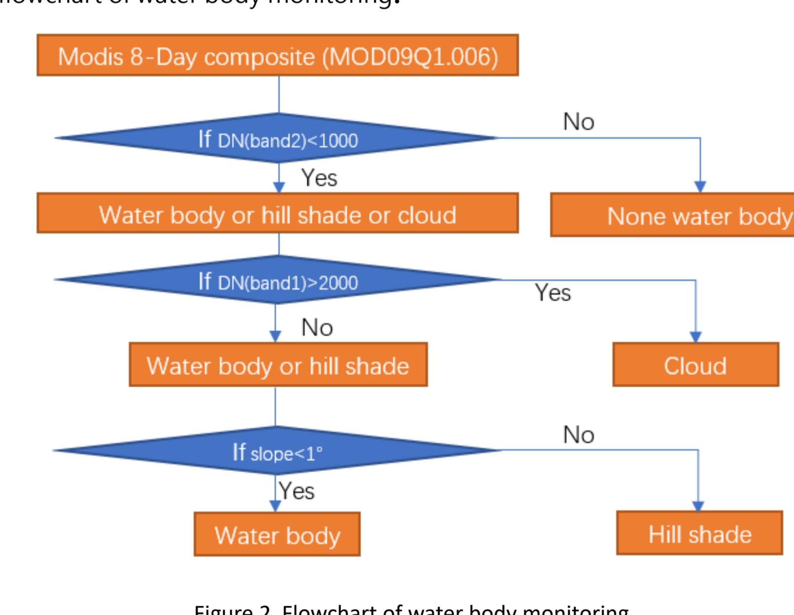
Figure 2 Flowchart of water body monitoring
