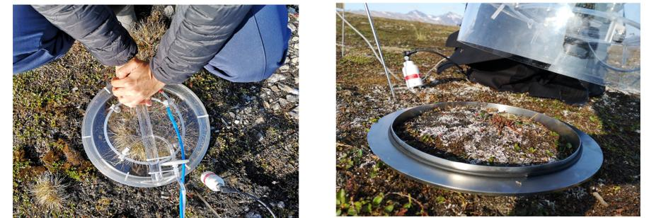
Fig. 8: The flux chamber in polymethyl-metachrylate, designed to have a high transmission coefficient of light in the visible spectrum, and how to insert it over the steel collar posed on the ground. The dark cover, soil temperature and moisture sensors are visible.
