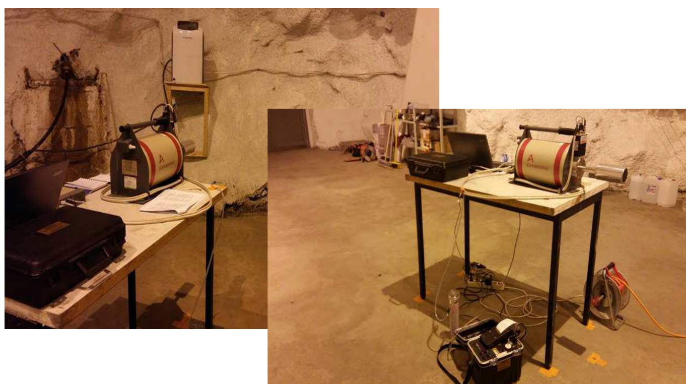
In-situ \gamma measurement (by using HPGe detector) and radon concentration in air (by using RAD7) at MP1
