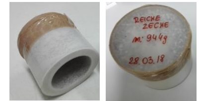
sample of rock placed in Marinelli container
