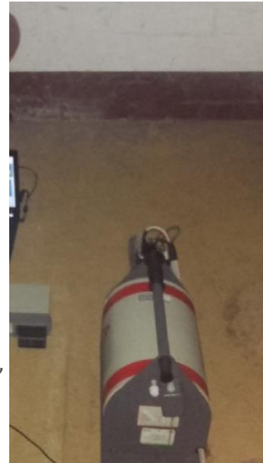
in-situ gamma ray measurement by using HPGe detector in server room
