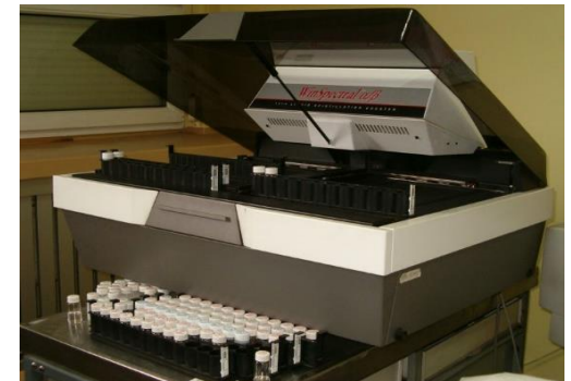
1414 WinSpectral \alpha/\beta LSC counter from Wallac
