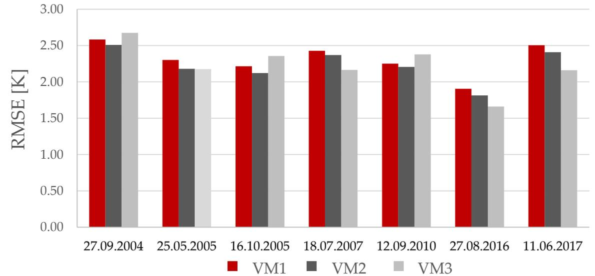
**Fig. 3.** Average Root Mean Square Error (RMSE) between enhanced images and reference images for VM1, VM2 and VM3 approaches
