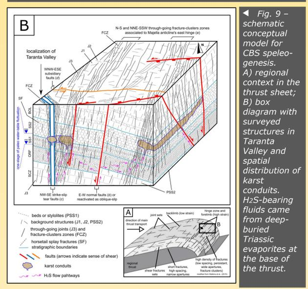
Fig. 9 - schematic conceptual model for CBS speleogenesis. A) regional context in the thrust sheet; B) box diagram with surveyed structures in Taranta Valley and spatial distribution of karst conduits. H<sub>2</sub>S-bearing fluids came from deep-buried Triassic evaporites at the base of the thrust.
