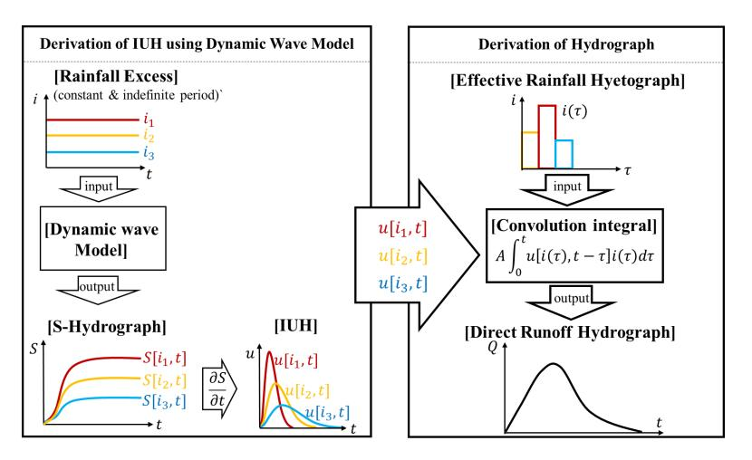
Schematic of dynamic wave based IUH (DIUH) method
