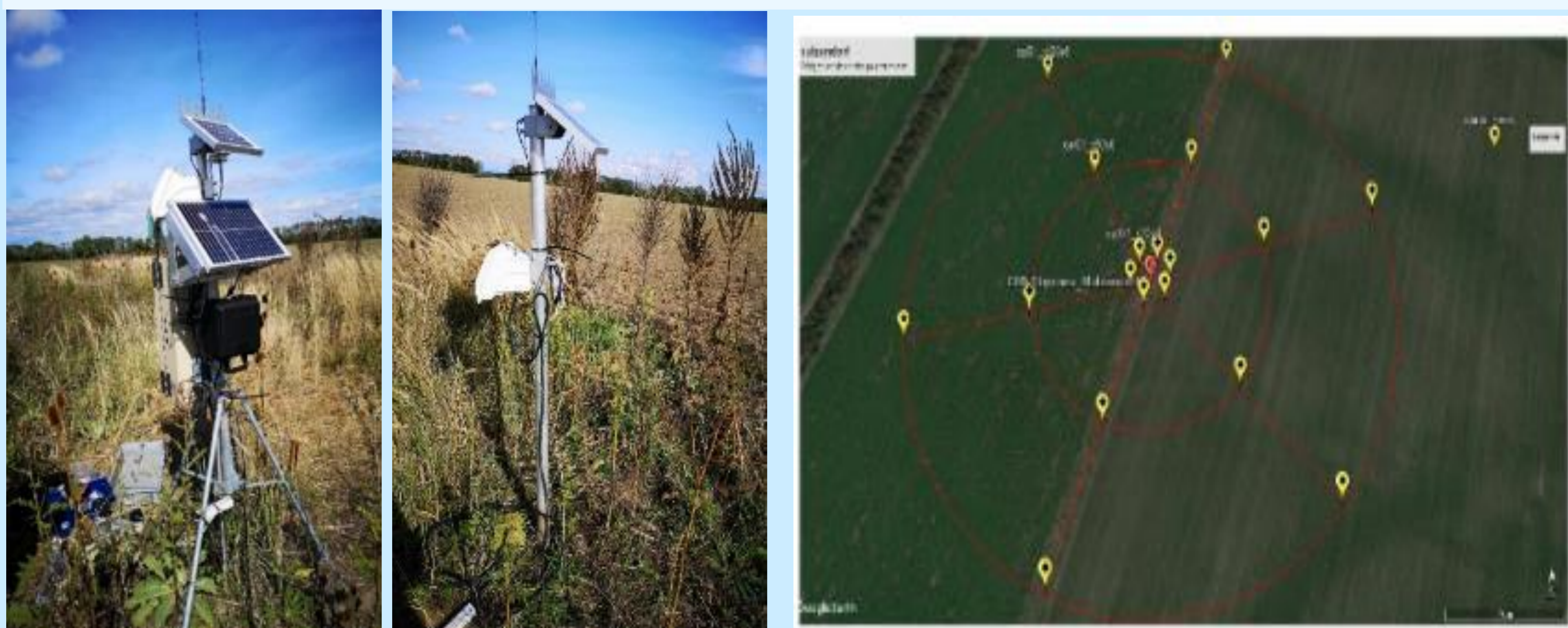
Fig.1 Cosmic Ray Neutron Sensor (left); Drill & Drop capacitance probe (right) installed in Rutzendorf Austria
