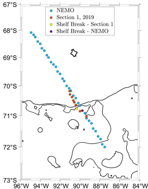
Figure 4: Map of picked cross-slope section for the NEMO Reanalysis data (blue dots) based on the location of the observed section 1 (red dots). The shelf break is defined for both of the sections (NEMO purple, Observation yellow).
