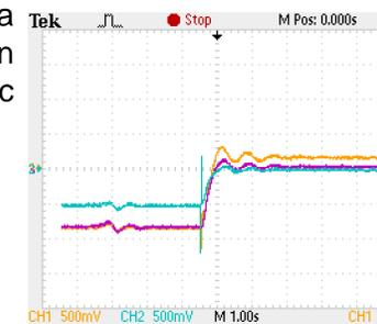
This oscilloscope screenshot shows the 3 capacitive position detectors behavior on the control loop start.
