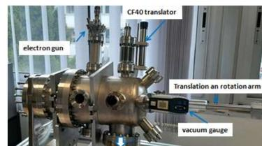
A floating metallic sample is put to a potential of -20V via the electron gun. Then the sample is lighted by a 240 nm UV LED. The current measurement is performed by the determination of the capacitance and the surface potential variation over time :
