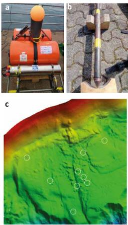
Figure 3: a) OBS - b) CPTu - c) Identification of OBS array geometry with multibeam bathymetry-
