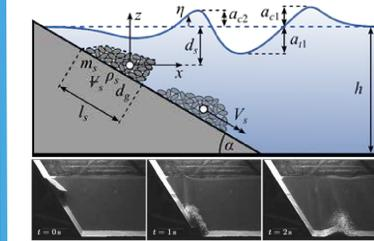
Figure 4: Wave generation by a subaqueous landslide in the VAW laboratory.
