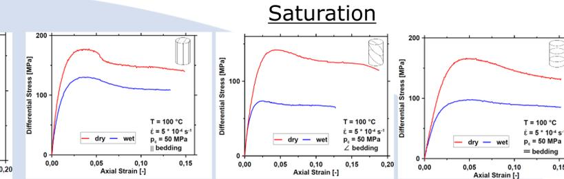
Fig. 4: Stress-strain curves showing the effect of saturation on the mechanical response of parallel, 45° and perpendicular oriented samples. Deformation conditions and sample orientation are indicated.
