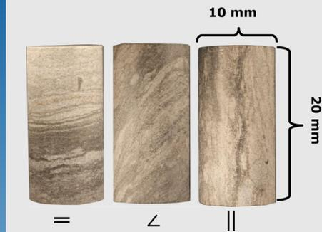
← Fig. 1: Sample cores prepared perpendicular, 45° and parallel to the bedding direction.
