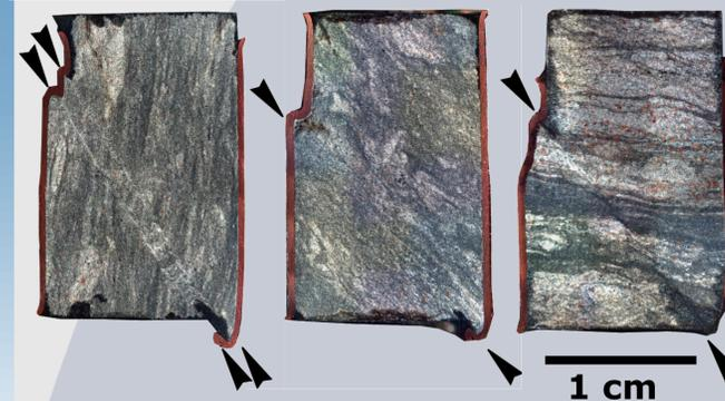
Fig. 5: Reflected light micrographs of typical deformation features in the Sandy facies of Opalinus Clay for dried samples deformed parallel (T=200 °C), 45° (T=25 °C) and perpendicular (T=200 °C) to the bedding direction. Black arrowheads indicate the traces of strain localization. Samples were deformed at  $p_c=50$  MPa and  $\dot{\epsilon}=5 \cdot 10^{-4} s^{-1}$ .
