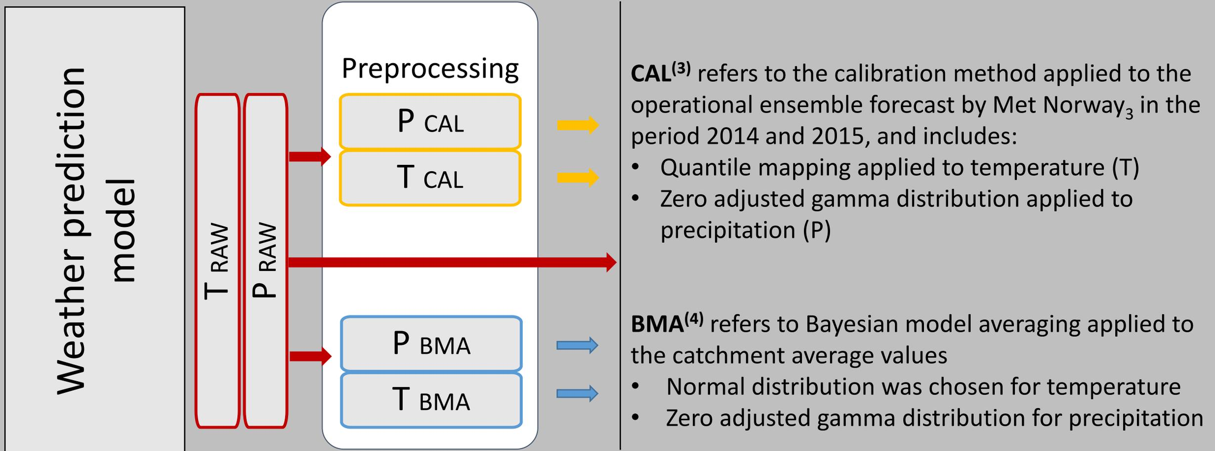
Combinations of T and P are forced the HBV models. Box-cox transformed streamflow is applied BMA, which enables an evaluation of the added effect of postprocessing
