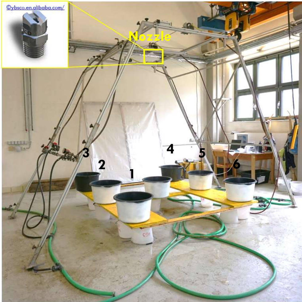
Rainfall simulator “BAW” with one FullJet nozzles with positions of splash cups marked with numbers.
