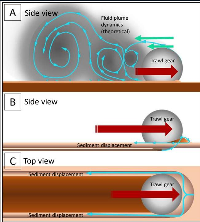
A] Trawl gears are a barrier to the flow of water, and as such will create friction between the gear surface and the water it is in contact with. Inflowing water is incrementally slowed by the slower plane below it, introducing turbulence in the wake of the gear.
