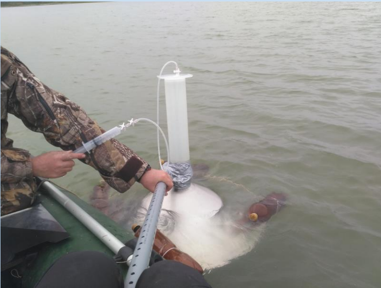
Seepage gas sampling
